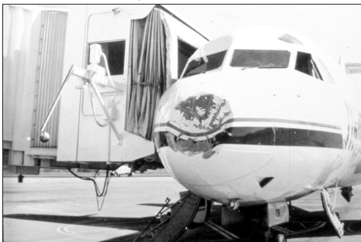
Figure 18. Just prior to landing at 50 feet above ground level, this aircraft struck a Red-tailed Hawk damaging the radome which disabled the navigation system. The passengers and crew experienced significant vibrations during landing. The pilot landed the aircraft safely, but emergency vehicles responded to ensure that mishaps did not occur.
